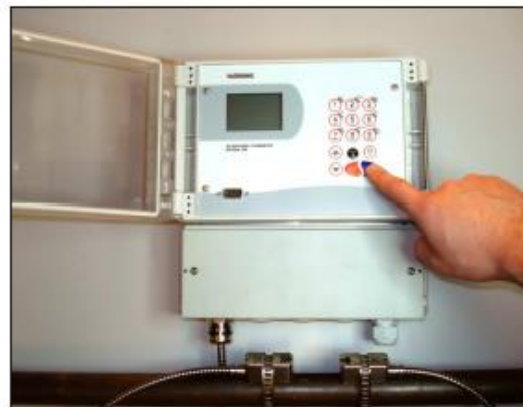
KATflow 150 wall-mounted with transducers
